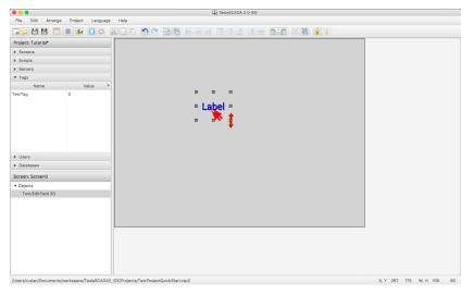
Screen you can see a graphical object **Text/EditField 3D** and squares for resizing graphical object. You can **Drag and Drop** these squares for resizing object.
