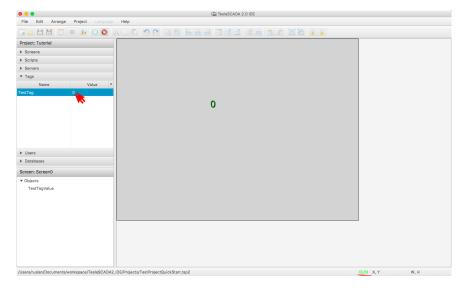
After starting simulation mode you'll see the RUN indicator in the lower right corner. Graphical object since we set up **Text Input** property displays default value **0**. To change tag's value **Double click** on the **TestTag** (we bound this tag to Text Input property) on the **Tags** pane.
