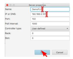
In the Server properties Dialog Box, type DemoPLC in the Name field to give the new server (your device) a name, in the IP or DNS type IP address of your device, then click OK.
