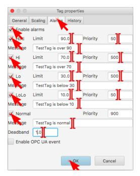
In the **Tag properties Dialog Box**, open **Alarms** tab by clicking on it. Check on **Enable Alarms**, **HiHi**, **Hi**, **Lo**, **LoLo** and **Normal** checkboxes. Fill up all **Edit boxes** like it's shown in the Picture. Then click **OK**.
