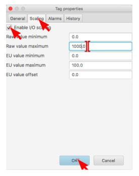
In the **Tag properties dialog box** open **Scaling** tab by clicking on it. Type 1000 in the **Raw value maximum** text field. Other text fields left unchangeable. Then click **OK.**
