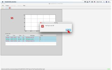
Because we set up **Alarms** in our **TestTag** we see Alarm message and in the **Event Log** new row is added.
