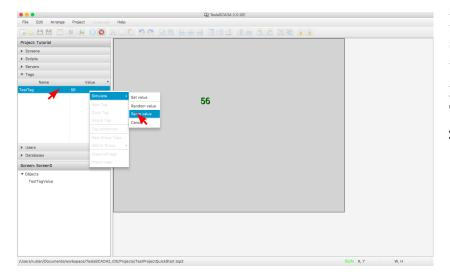
It is also possible to simulate a sequential change in the tag's value from 0 to 100. To do this you should **Right Click** on the **TestTag** and choose **Simulate->Ramp** menu item.
