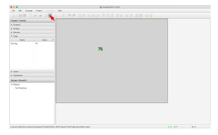
To stop **Simulation mode** on the Tool Bar, click on the **Stop simulation** icon.
