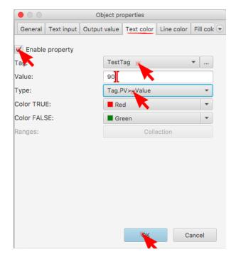
On the **Text color** tab check **Enable property**. Choose **TestTag**, **Type 90** in the **Value** field and Choose **Tag.PV>=Value** in the **Type** ComboBox.
